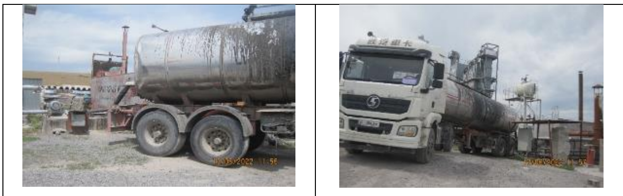
Figure 58 Refueling of asphalt plant tanks with bitumen by bitumen trucks
