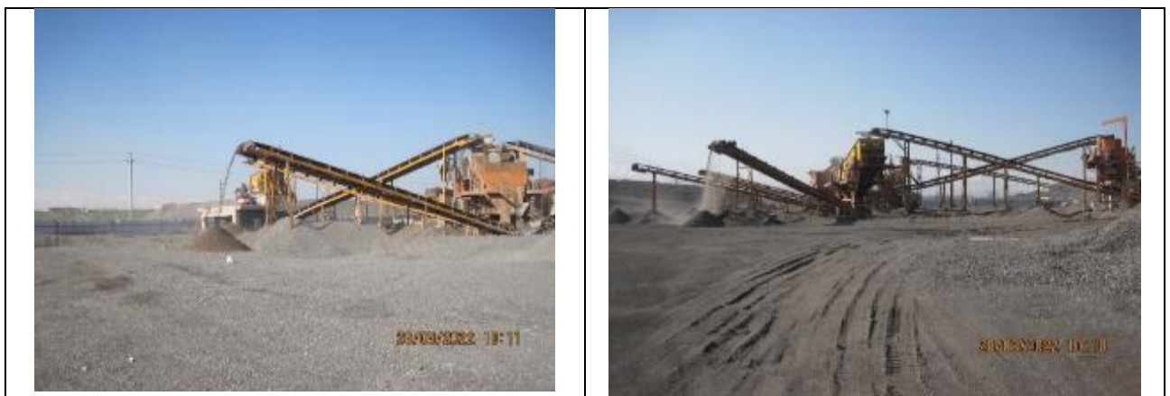
Figure 38 Operation of a stone crushing plant on moistened raw materials
